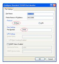
Click "OK", then "Next" to complete the setup. Then the wizard will prompt you to select the printer driver to associate with this TCP printer port. Choose the printer model accordingly.
